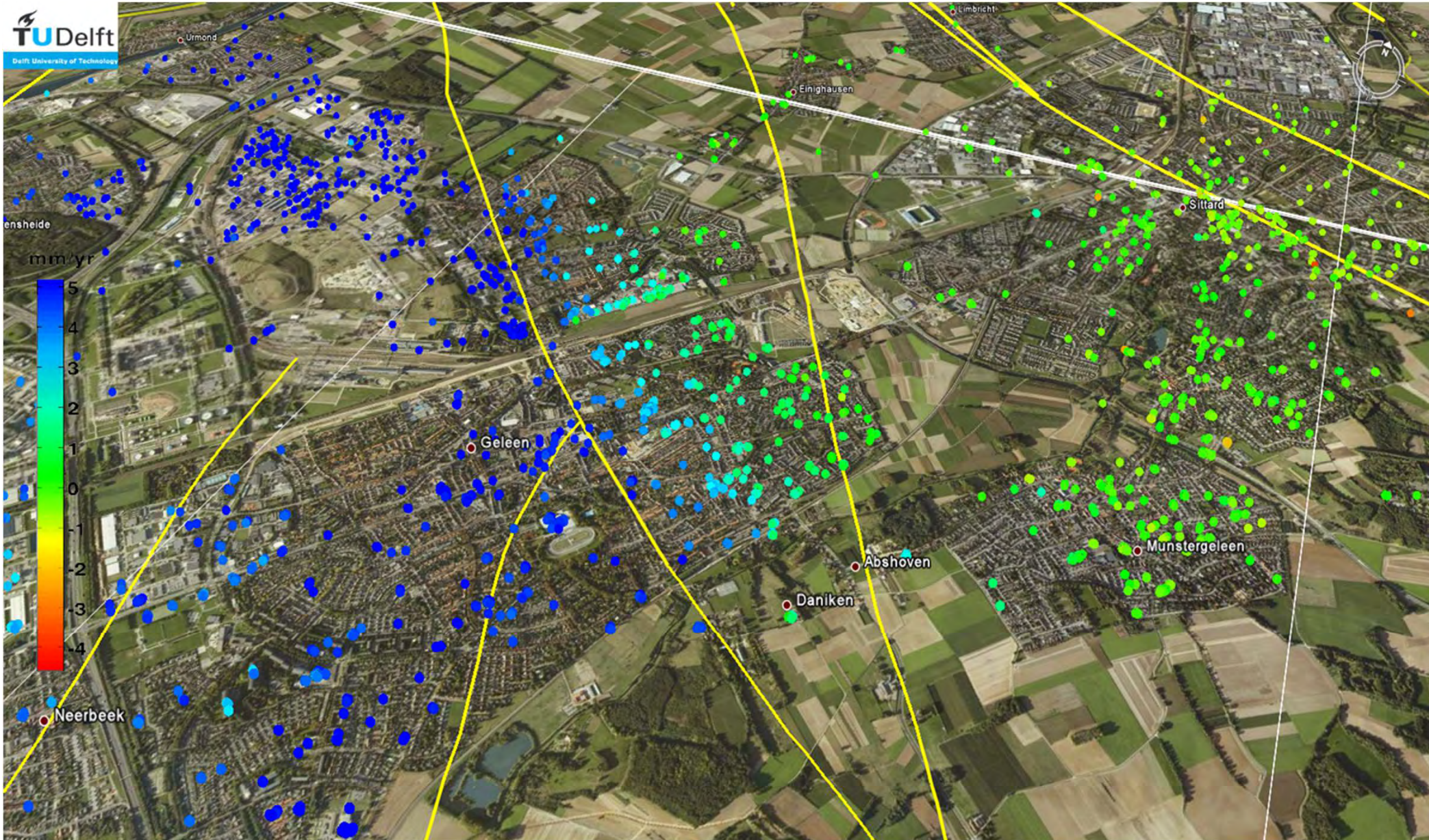
InSAR picture with differential movements Heerlerheide breuk (TU Delft)
