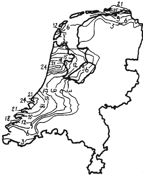
Figure 13 Depth of top of Pleistocene sediments in m-NAP (After Zagwijn et al., 1985).
