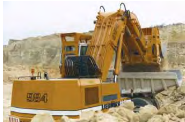
Figure 9. Shovel loading the dump truck in the calcarenite, open pit south of Maastricht (N° 2, figure 1). (Photo: Courtesy of ENCI, Maas-
