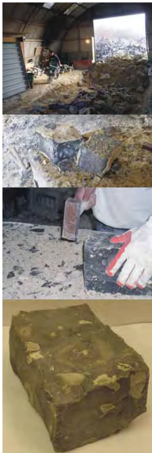
Figure 10. Modern silex exploitation. The silex is mined near Eben-Ezer (N° 11, figure 1). The silex is chiselled by manual labour into prism shaped brick. These bricks (masonry) are used as silex tube mill liner. Length: 14cm to 13.5cm; width: 9.5 to <9cm; height: 6.5 to 6.7cm. In the 20 th century the silex was still mined underground in galleries. Today the silex is provided by the open pit (N°5; figure 1). (Photo: Autumn 2004)
