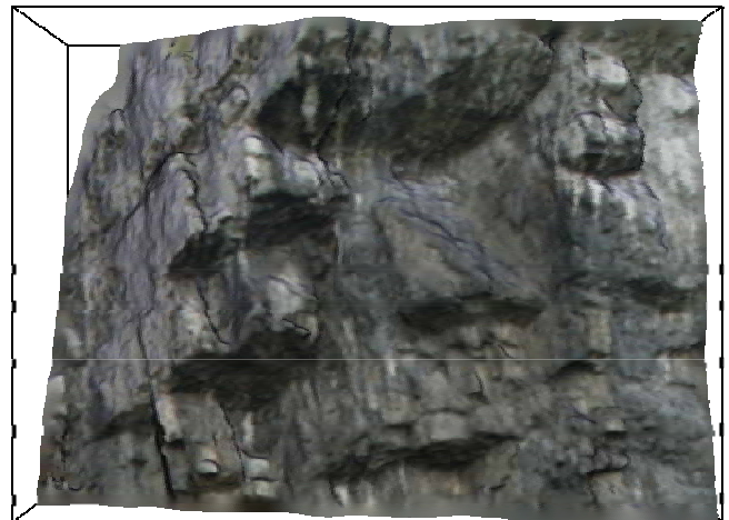
Figure 6. This is the same 3D rendered surface model as Figure 3. Instead of using artificial illumination, in this case each facet in the 3D surface has been coloured using the colour information from the point cloud.
