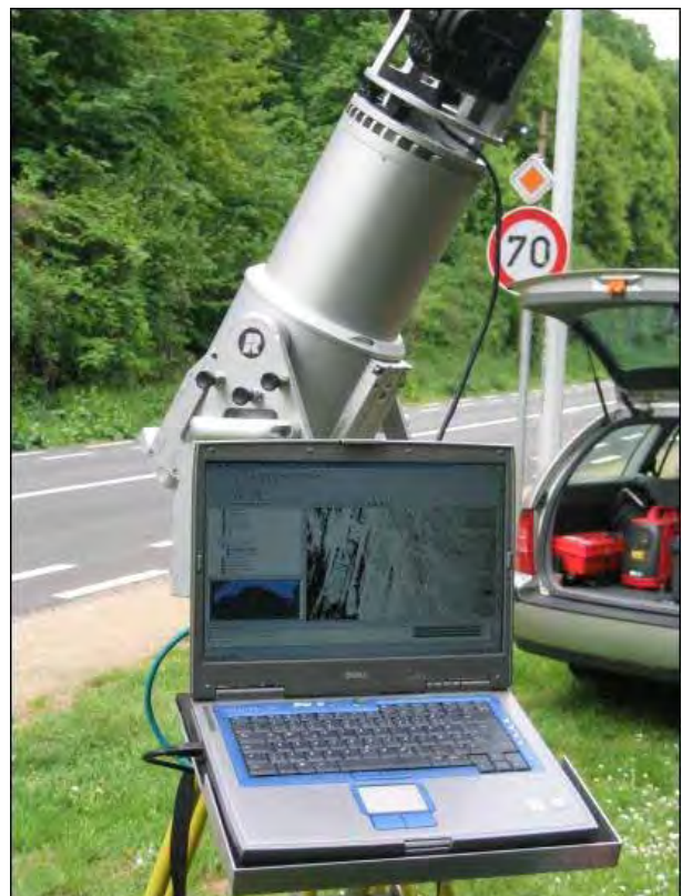
Figure 2. The 3D laser scanner (Riegl 3D Imaging Sensor LMS-Z420i) in action. You can see that the point cloud data that has just been generated can be visualised in real-time. Note the high resolution digital camera mounted on top. The laser is slightly tilted to accommodate the entire slope in one scan.
