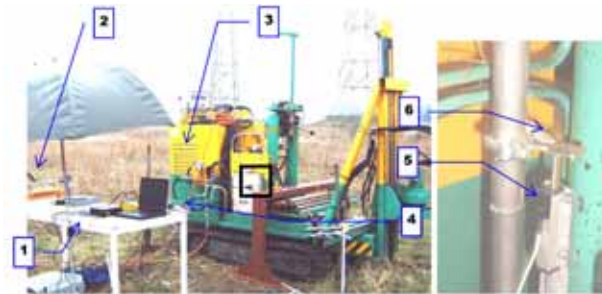
Fig. 8 Cone load test set-up: 1) device used to visualise and record the parameters during the cone load tests and penetration, 2) pump, 3) connection of the hand pump on the hydraulic system of the CPT, 4) rigid structure anchored in the ground, independent of the thrust machine, 5) displacement transducer, 6) plate attached to the push rods for measurement of displacements
