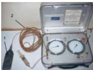
Fig. 10 Marchetti dilatometer probe (top) and pressure control and read-out unit (bottom)
