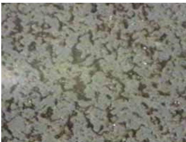
Fig. 5 Creosote oil in the subsoil as seen by the video cone (image size is 5x7mm)
