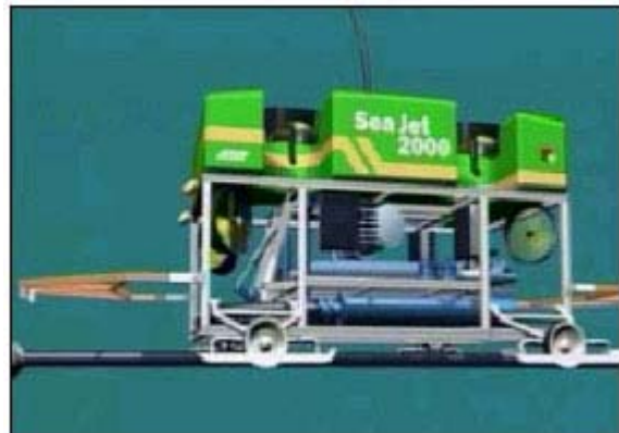
Figure 3. Seajet aligned along pipeline
