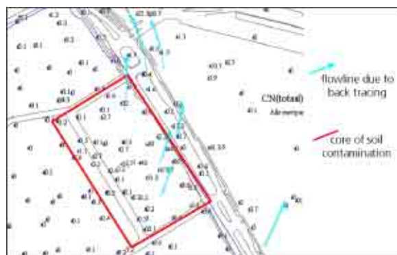
Figure 4: Back tracing along flow lines. The flow lines (light blue lines) end at the depth of the observation well at which the concentration level exceeds more than five times the Dutch intervention level for cyanide. The flow line starts at the groundwater table where replenishment with infiltrating rainwater takes place.
